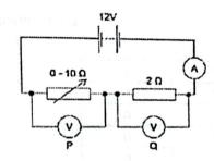
Which graph shows the variation with current of the voltmeter readings?
