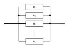
$$R_{eff} = \left(\frac{1}{R_1} + \frac{1}{R_2} + \frac{1}{R_3} + \dots + \frac{1}{R_n}\right)^{-1}$$
