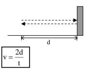
v: speed of sound [m/s] d: **one-way** distance [m] t: time taken for echo to be received [s]
