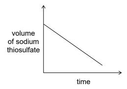
The volume of  $Na_2S_2O_3$  used for titrating a sample of quenched aliquot at time t is proportional to the concentration of  $I_2$  present in the reaction mixture at time t.
