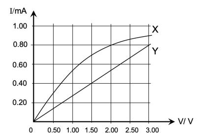
Two components X and Y are connected in parallel with a 3.0 V battery. What is the amount of energy used in the battery in 1.5 minutes?
