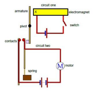
If the current flowing in the electromagnet is decreased, which of the following changes should be made to the circuit such that the motor can still be turned on when the switch is closed?
