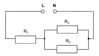
What is the ratio of power dissipated by R<sub>1</sub>, R<sub>2</sub> and R<sub>3</sub>?
