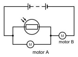
When the lights in the room are switched off, what would happen to the speed of motors A and B?
