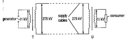
In order to do this, the electricity supply company makes use of a circuit containing two transformers T and U. The transformers can be considered to be ideal and the supply cables to have negligible resistance.
