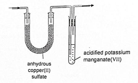
The student observed that the white anhydrous copper(II) sulfate turned blue and the purple acidified potassium manganate(VII) turned colourless.
