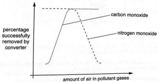
(i) Describe and explain how increased amounts of air affect the removal of carbon monoxide and nitrogen monoxide.
