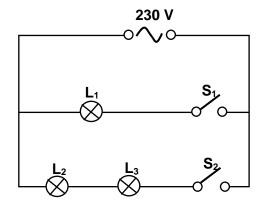
What is the current flowing through  $L_3$  when the switches  $S_1$  and  $S_2$  are closed?
